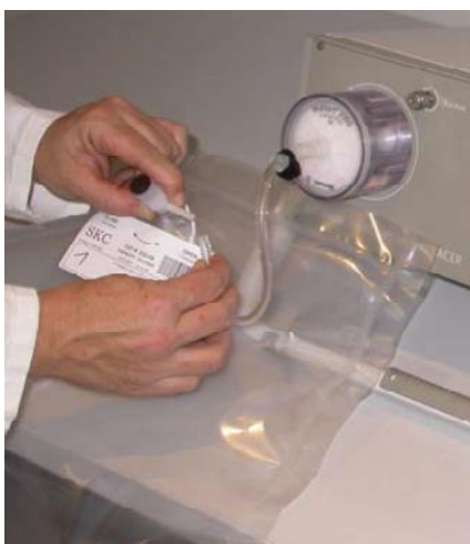
Connecting a Tedlar® bag filled with sample to the UT-3000
