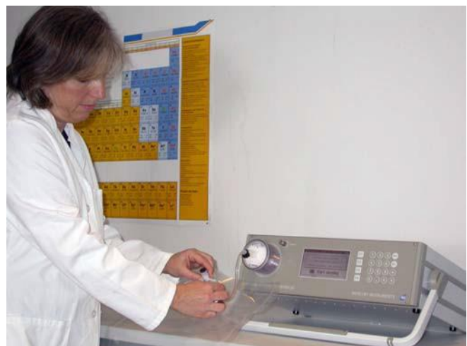
Opening of the valve to release sample into the analyzer
